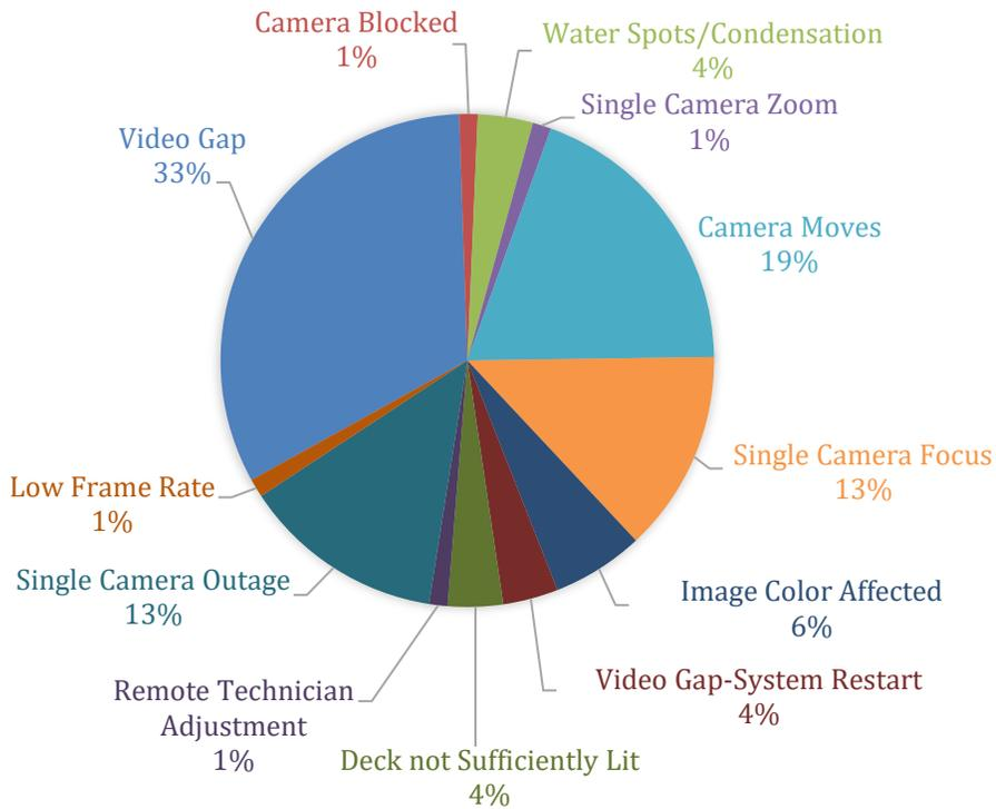
couplers. Finally, video gaps comprised 37% of EM malfunctions identified, with 4% resulting from an EM system restart. Video gaps not caused by a system restart were most often caused by fluctuations in power to the EM system, and could usually be resolved following a trip by switching the system power source or improving connections between the EM system and the vessel power.
